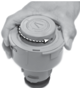
Fig. 9: To unlock turn tool clockwise
